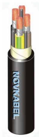
**Flexible cable for submersible pumps****Standard:** PSN**Nominal voltage  $U_0/U$ :** 0,6/1 kV**Test voltage:** 2,5 kV**CONSTRUCTION****Conductor:** flexible copper conductor class 5.**Insulation:** based on EPR rubber.**Inner sheath:** based on synthetic rubber (if exists).**Sheath:** specially adapted compositions based on rubber. Sheath colour black.**APPLICATION**
